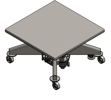
360° CONTINUOUS DECK ROTATION. LOCK IN PLACE AT ANY LOCATION WITH AIR REGULATOR, FILTER, LOCK HANDLE LUBRICATOR-0.25 THICK FORMED STEEL DECK PLATE DECK ROTATION 27.00 LOCK HANDLE LOWERED -AIR MOTOR, (18.00 TRAVEL, 80 PSI, 50 CFM 45.00 RAISED)
